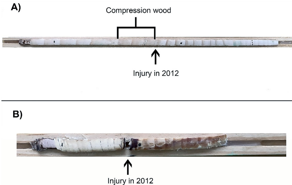
Figure 5 Increment cores with growth disturbances caused by the 2012 lahar. In both examples, some marks corresponding to the dating performed can be observed. In each case, these marks, from right to left, refer to the years 2010 and 2020, respectively. A) Compression wood that began to grow the year following the lahar event, specifically, in 2013. Its main characteristic is an increase in wood production, which usually appears as larger growth rings with a darker coloration. B) The injury was dated in the late-late wood of 2012.
