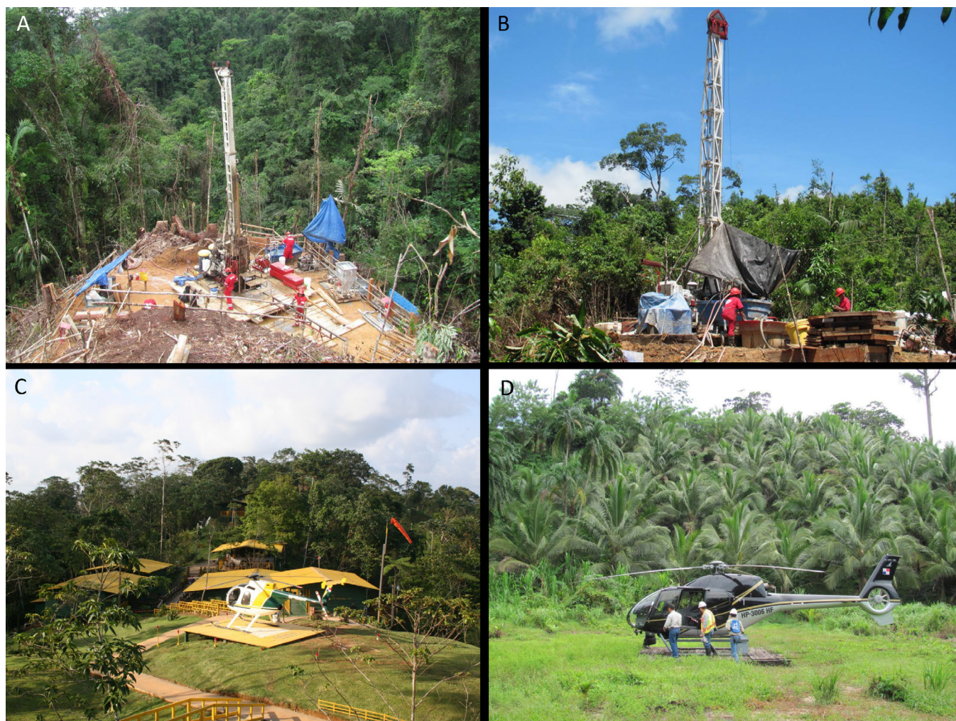
Figure 19 Exploration at Cobre Panama by Minera Panama S.A. in 2007-2011. A) Diamond drilling at Botija Abajo with a Boart-Longyear LF-70 rig, June 2010. B) Diamond drilling at Balboa with a Boart-Longyear Fly 38 rig, October 2011. Both drills were portable and all of the drilling was carried out by helicopter slinging. C) Colina camp with a Hughes 500 helicopter, 18 March 2007. D) Eurocopter Colibri helicopter pickup of a community relations field party at Rio Caimito, October 2010. (Photographs A, B and D by Colin Burge. Photograph C by Stewart Redwood).
