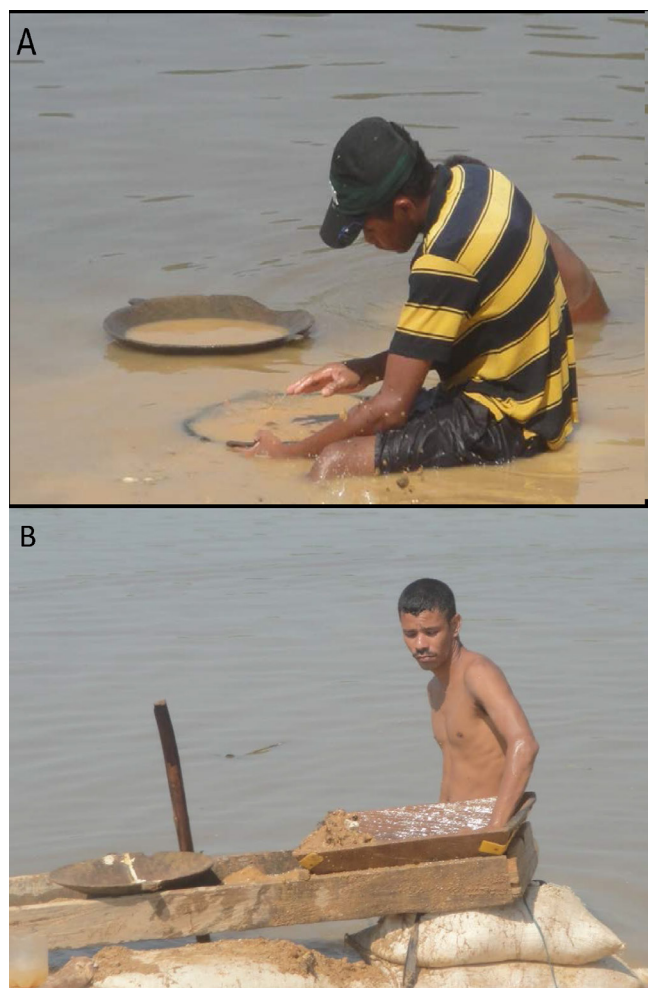
Figure 10 Wooden, two-handed bateas in use today at the Santa Cruz mine on the Rio Magdalena, Bolivar, Colombia. In B) the batea is being used to clean up the concentrate from a sluice. The batea was probably used by indigenous miners in the Caribbean and Mesoamerica before the Spanish arrival. (Photographs by Stewart Redwood, 25 January 2012).
