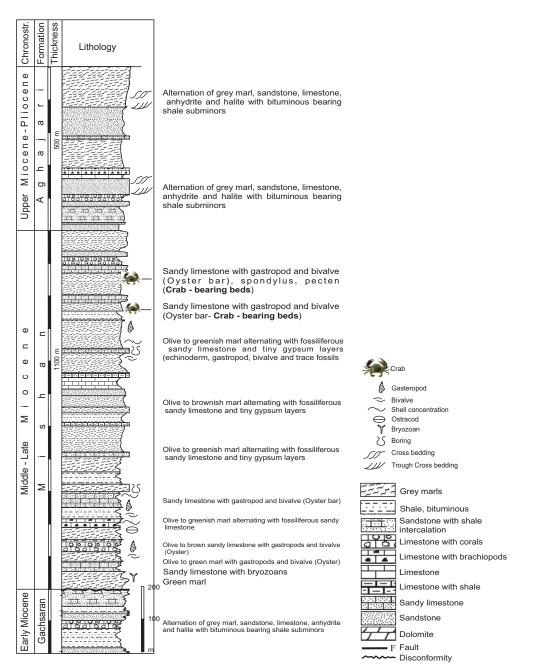
Figure 1. Composed stratigraphic column at Konar Takhteh and Ahram sections, Southern Iran, with position of crustacean-bearing horizons of the Mishan Formation.
